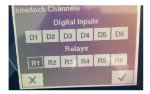
Since the R1 menu has Interlock Channels R4, and the R4 menu has Interlock Channels R1, whichever relay activates first will prevent the other relay from activating. This is referred to as Mutual Interlock.
