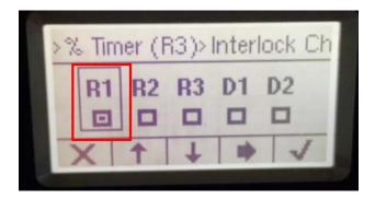
Since the R1 menu has Interlock Channels R3, and the R3 menu has Interlock Channels R1, whichever relay activates first will prevent the other relay from activating. This is referred to as Mutual Interlock.
