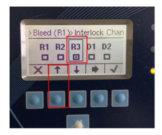
In the above example, you've programmed the R1 relay such that if R3 activates, R1 will be interlocked. If R1 is On when R3 activates, R1 will immediately shut Off. If R1 is Off when R3 activates, R1 will not be able to activate until R3 deactivates. This is referred to as Permissive Interlock.
