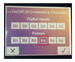
In this example, you've programmed the R1 relay such that if R4 activates, R1 will be interlocked. If R1 is On when R4 activates, R1 will immediately shut Off. If R1 is Off when R4 activates, R1 will not be able to activate until R4 deactivates. This is referred to as Permissive Interlock.
